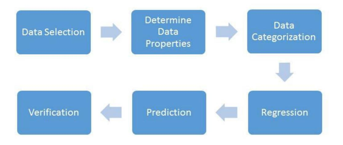
Modeling for CBM is a data-dependent process. Data acquisition, processing, and required for modeling analysis the are behavior of the "normal" operating conditions of the diesel engine. This thesis leverages on existing data collected through sensors on a diesel engine to describe these conditions using regression analysis. The proposed data selection criteria ensure that data used for modeling are suitable.
