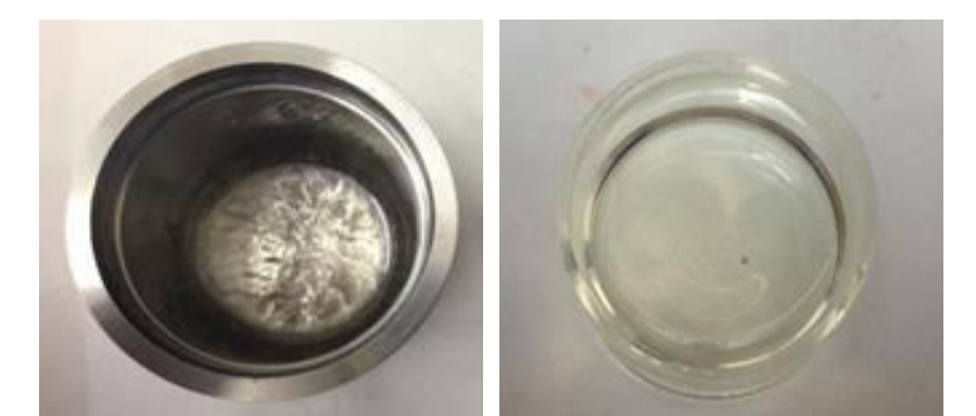
(L) Two-phase followed by (R) single phase liquid after 5 min of pre-mixing
