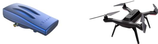
**3DR Solo Drone** is the principal mode of platform employed for the field-based effectiveness testing. The platform is a quadcopter design with four motor pods, compass, antenna, GPS, and electronic speed controllers and propellers. Furthermore, its mainboard computer has the capabilities to control navigation, attitude, and communication.
