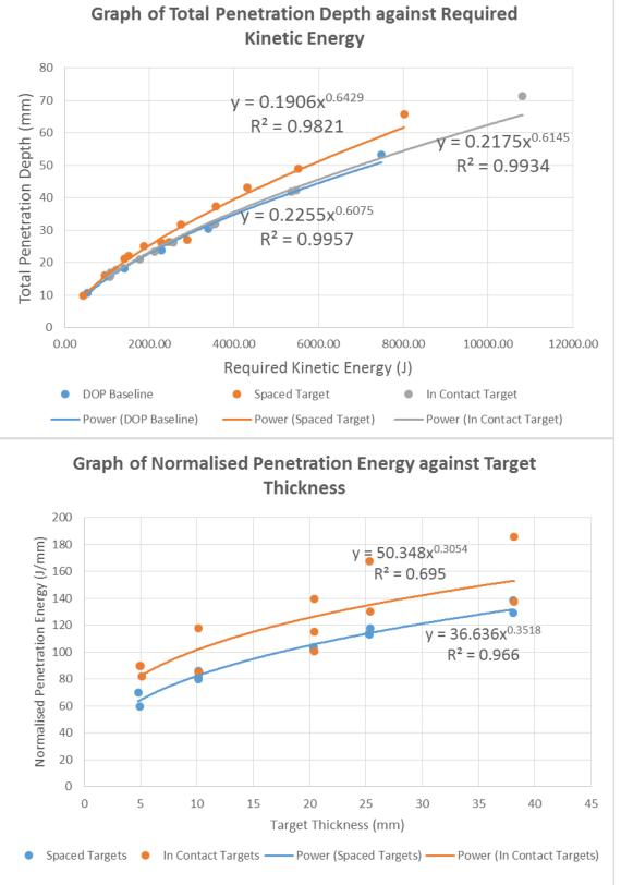
• In-contact targets required approximately 20% higher kinetic energy for penetration, and appeared to have ballistic similar displayed performance characteristics to a monolithic block.
