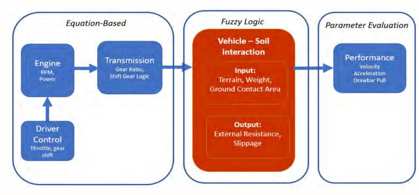
• Equation-based Powertrain Model premised on equation of motion with data from engine performance, driveline gear ratio, gear shift logic and wheel parameter.
