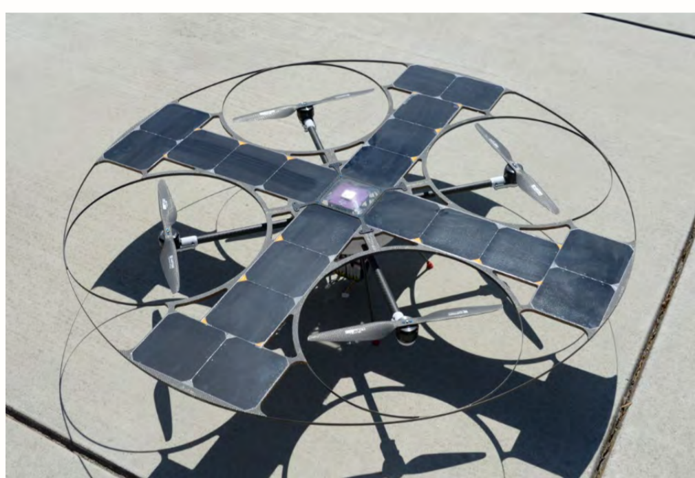
Aqua-Quad Quadrotor Prototype (1.1 x 1.1 m, ~3.5 kg)
