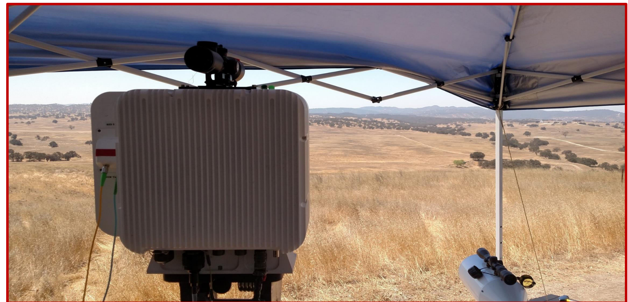
NEXUS 3 FSO communications system, 9.40km link, Camp Roberts
